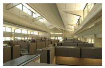
**PORT HUENEME, CA** Navy Building 850 at Naval Base Ventura County (NBVC) incorporated energy efficient design elements, including skylights, open ceilings, exposed ventilation system ductwork, which maximizes the use of natural ventilation, and 100 percent daylighting. The building employs energy saving equipment, including energy efficient lighting and HVAC systems. Together, these features earned the building an outstanding ENERGY STAR® benchmarking score of 96.
