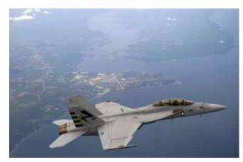
**PATUXENT RIVER, MD** An F/A-18F Super Hornet strike fighter, dubbed the "Green Hornet," conducts a supersonic test flight. The aircraft is fueled with a 50/50 blend of biofuel and conventional fuel. (U.S. Navy photo by Liz Goettee)
