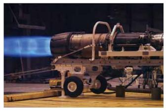
**PATUXENT RIVER, MD** An F404 engine from an F/A-18 runs on biofuel in a Naval Air Systems Command test at the Aircraft Test and Evaluation Facility, Patuxent River, MD. *(U.S. Navy photo by David Sckrabulis)*
