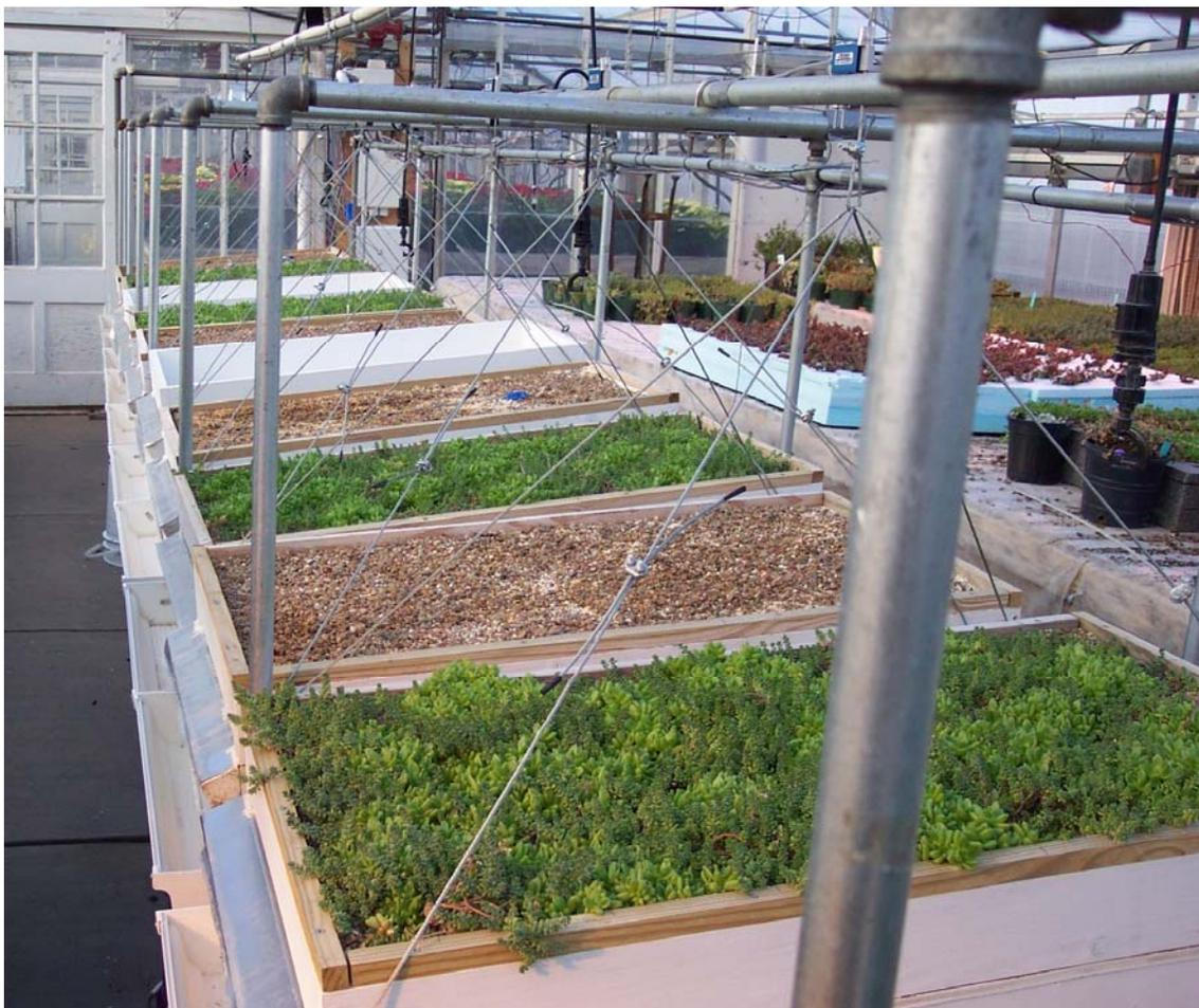
Figure A-1. Model green roof test beds suspended from load cells, lysimeters studies, in Penn State University greenhouse for evapotranspiration studies
