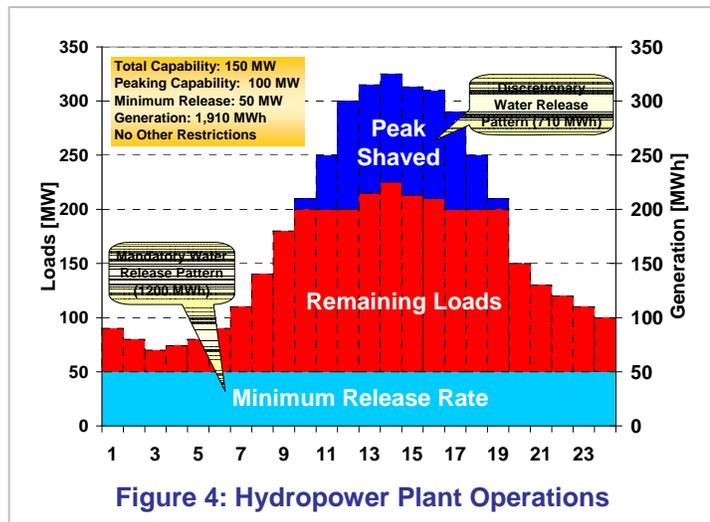
Figure 4: Hydropower Plant Operations
