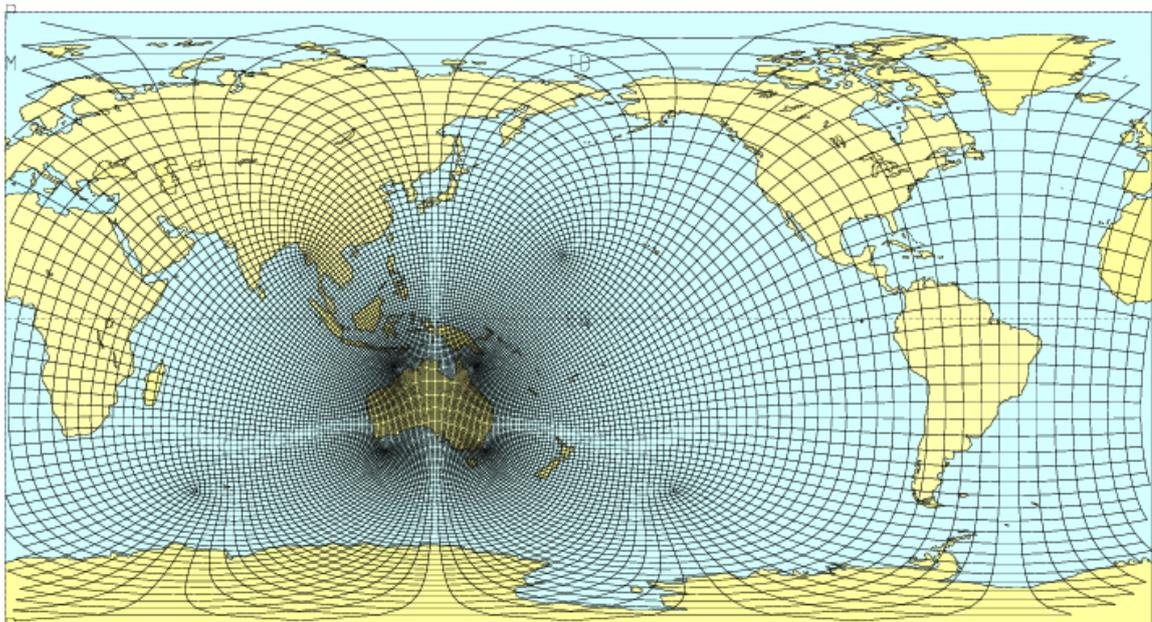
Figure 2: Diagram illustrating the stretched grid of the cubic conformal model.
