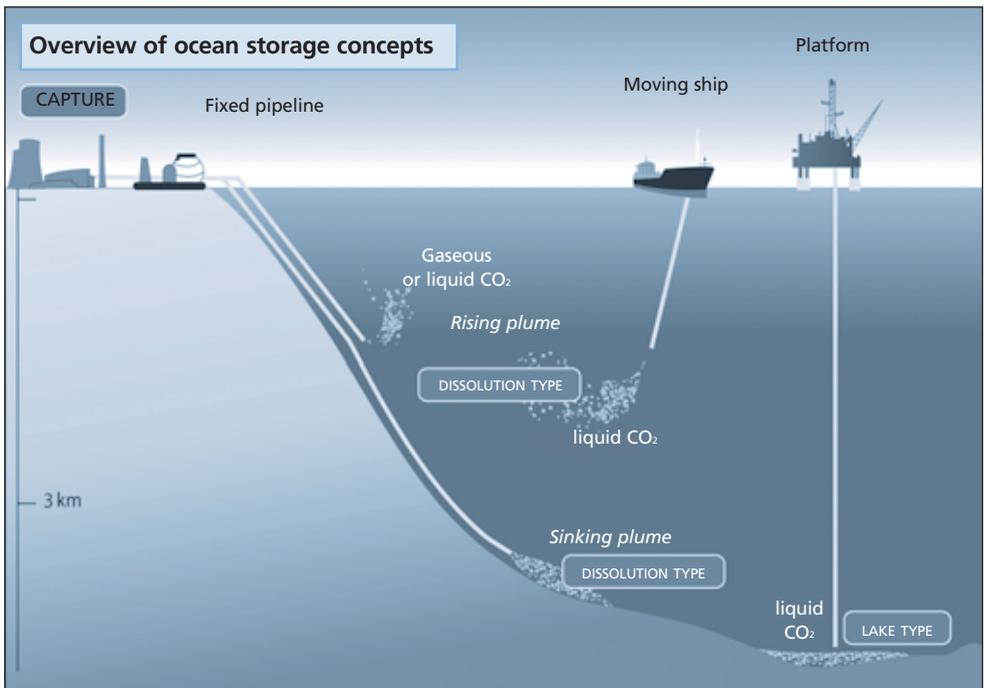
can be released into the ocean water column via a fixed pipeline or from a moving ship. Alternatively, it can be deposited onto the deep seafloor at depths below 3,000m, where CO<sub>2</sub> is denser than water. These technologies, however, are still in the research phase, have not undergone full-scale testing and could have negative impacts on the ocean environment.
