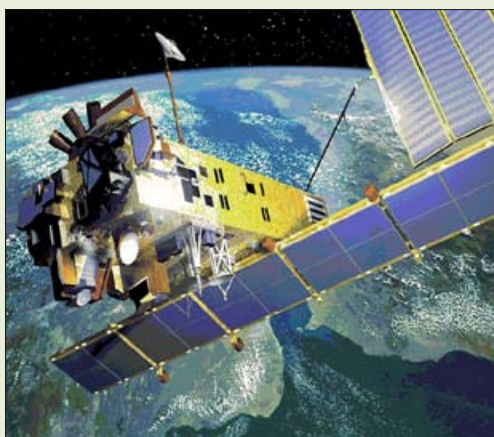
Figure B2.4. ENVISAT, a European satellite providing continuous observations of the Earth including measurements related to atmospheric chemistry, sea surface temperature and ice coverage.
