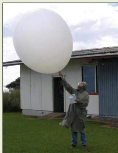
Figure B2.2. Releasing a hydrogen-filled balloon with a radiosonde attached – Lord Howe Island
