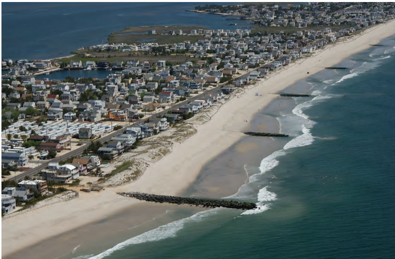
Figure 4. Oblique aerial photograph showing an extensive groin field at Beach Haven, NJ. Groin fields such as this are common in many parts of New England and the Mid-Atlantic. Photograph is taken looking to the northwest.
