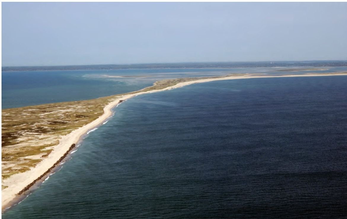
Figure 17. Oblique aerial photograph of Monomoy Island, MA, where the maximum long-term erosion ( -12.1 meters per year) and accretion ( 8.1 meters per year) rates in the Cape Cod region were measured. The photograph is looking to the north.
