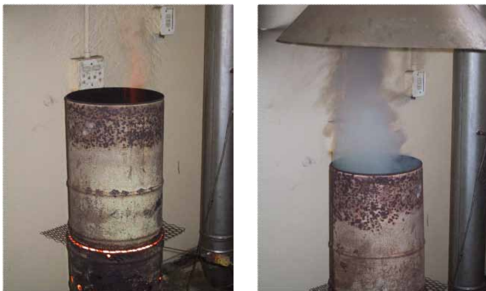
Figure 5.5. Basa njengo Magogo: Comparative smoke emissions from the Basa njengo Magogo fire (left) and a fire ignited with the bottom-up method (right), using traditional D-grade coal. (Source: CSIR Environmentek (2005))
