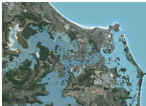
Figure 5.12 Images of Tweed Heads in 2009 and with simulated inundation from a sea-level rise of 1.1 metres and a 1-in-100 year storm tide using medium resolution elevation data (not suitable for decision-making). © CNES 2009 / imagery supplied courtesy of SPOT Imaging Services and Geospatial Intelligence PTY LTD
