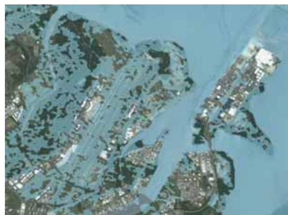
Figure 5.48 Images of Brisbane airport in 2009 and with simulated inundation from a sea-level rise of 1.1 metres using medium resolution elevation data (not suitable for decision-making). © CNES 2009 / imagery supplied courtesy of SPOT Imaging Services and Geospatial Intelligence PTY LTD
