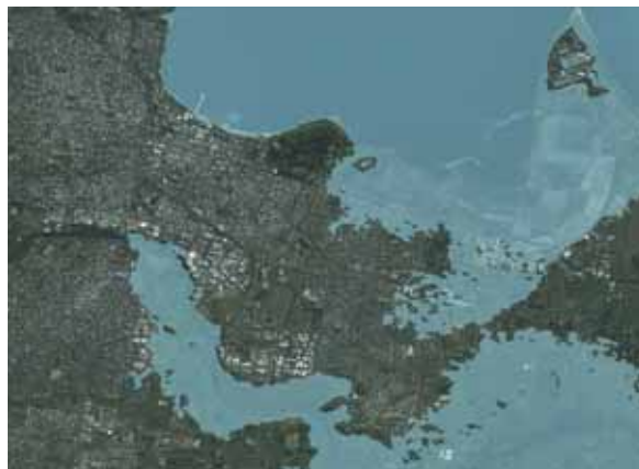
Figure 5.26 Images of Geelong (Greater Geelong LGA) in 2009 and with simulated inundation from a sea-level rise of 1.1 metres and a 1-in-100 year storm tide using medium resolution elevation data (not suitable for decision-making). © CNES 2009 / imagery supplied courtesy of SPOT Imaging Services and Geospatial Intelligence PTY LTD
