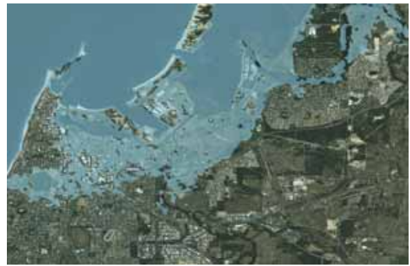
Figure 5.44 Images of Bunbury in 2009 and with simulated inundation from a sea-level rise of 1.1 metres using medium resolution elevation data (not suitable for decision-making). © CNES 2009 / imagery supplied courtesy of SPOT Imaging Services and Geospatial Intelligence PTY LTD.
