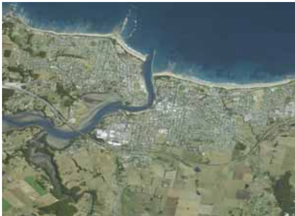
Figure 5.32 Images of Ulverstone in the Central Coast LGA in 2009 and with simulated inundation from a sea-level rise of 1.1 metres and a 1-in-100 year storm tide using medium resolution elevation data (not suitable for decision-making). © CNES 2009 / imagery supplied courtesy of SPOT Imaging Services and Geospatial Intelligence PTY LTD.
