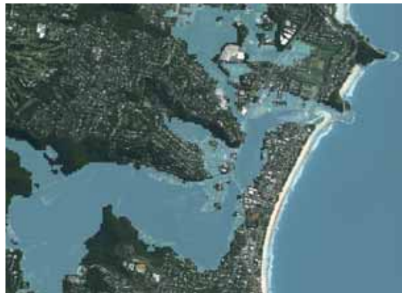
Figure 5.11 Images of Narrabeen/Collaroy (Pittwater LGA) in 2009 and with simulated inundation from a sea-level rise of 1.1 metres and a 1-in-100 year storm tide using medium resolution elevation data (not suitable for decision-making). © CNES 2009 / imagery supplied courtesy of SPOT Imaging Services and Geospatial Intelligence PTY LTD
