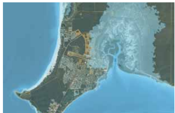
Figure 5.45 Images of Broome in 2009 and with simulated inundation from a sea-level rise of 1.1 metres using medium resolution elevation data (not suitable for decision-making). © CNES 2009 / imagery supplied courtesy of SPOT Imaging Services and Geospatial Intelligence PTY LTD.
