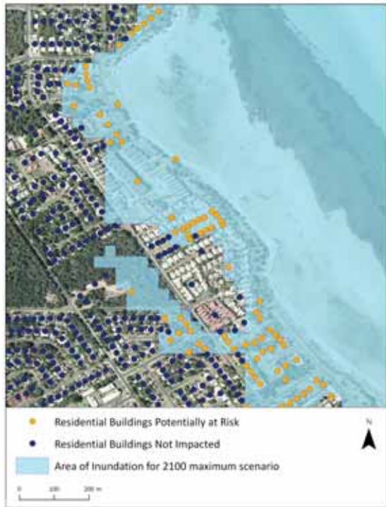
Figure 3.8 Example of overlay of NEXIS with an inundation footprint. Source: Geoscience Australia 2009
