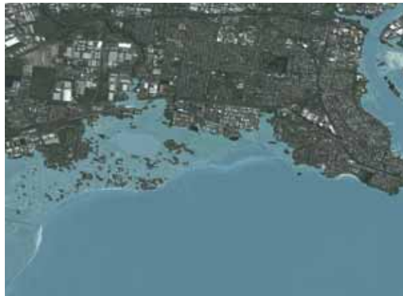
Figure 5.25 Images of Altona (Hobsons Bay LGA) in 2009 and with simulated inundation from a sea-level rise of 1.1 metres and a 1-in-100 year storm tide using medium resolution elevation data (not suitable for decision-making). © CNES 2009 / imagery supplied courtesy of SPOT Imaging Services and Geospatial Intelligence PTY LTD
