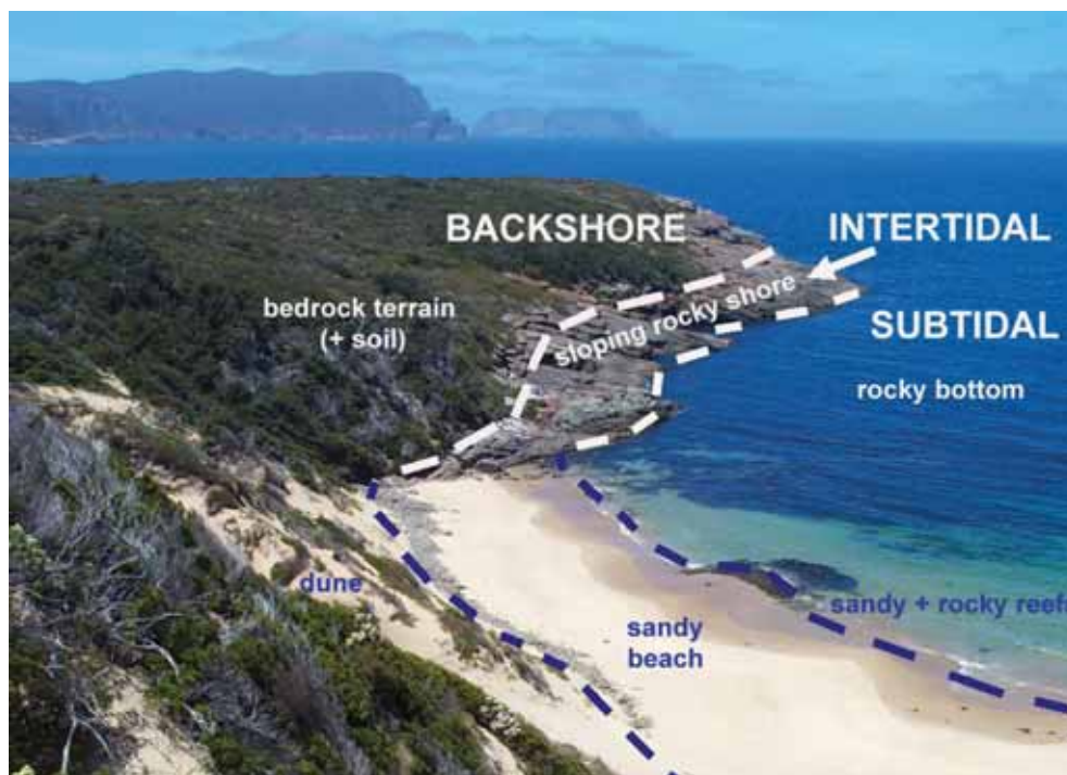
Figure 3.2 Illustration of the coastal attributes captured in the National Coastal Geomorphology Mapping tool. Source: Sharples et al. 2009 4
