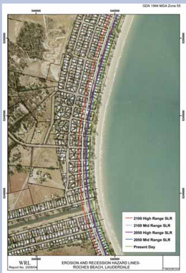
Figure 5.34 Erosion and recession hazard lines along the central section of Roches Beach. Source: Water Research Laboratory, UNSW
