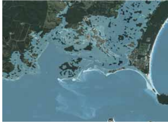
Figure 5.10 Images of Port Stephens in 2009 and with simulated inundation from a sea-level rise of 1.1 metres and a 1-in-100 year storm tide using medium resolution elevation data (not suitable for decision-making). © CNES 2009 / imagery supplied courtesy of SPOT Imaging Services and Geospatial Intelligence PTY LTD
