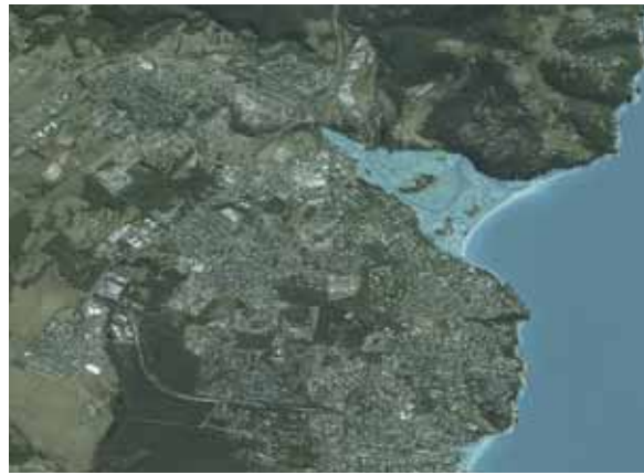
Figure 5.31 Images of Kingston (Kingborough LGA) in 2009 and with simulated inundation from a sea-level rise of 1.1 metres and a 1-in-100 year storm tide using medium resolution elevation data (not suitable for decision-making). © CNES 2009 / imagery supplied courtesy of SPOT Imaging Services and Geospatial Intelligence PTY LTD.
