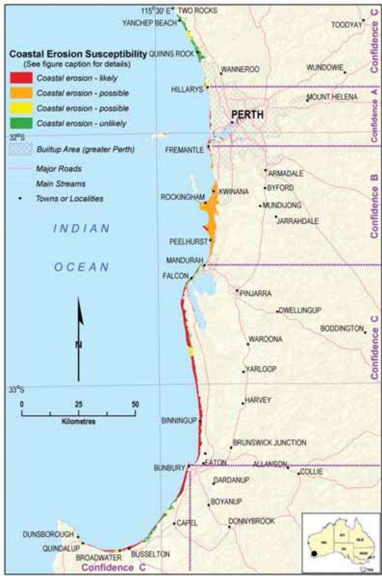
Figure 5.46 Coastal erosion susceptibility in Perth. Source: Jones 2005 164
