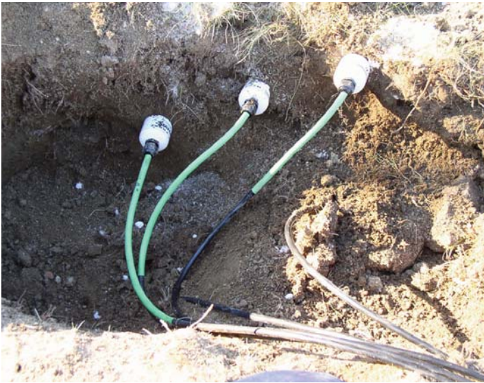
The pit in which the soil moisture probes have been installed to measure soil moisture over three different depths
