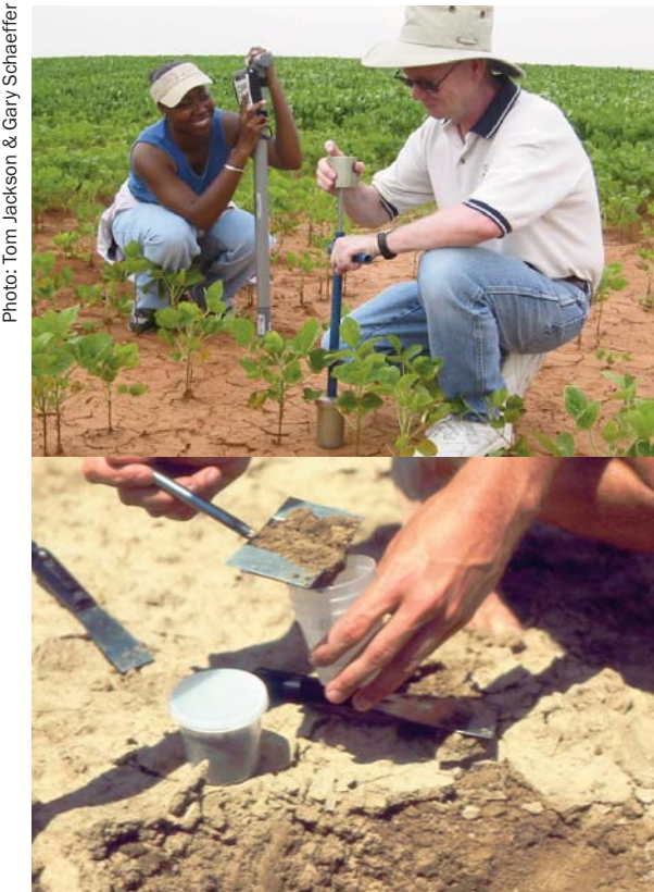
The measurement of soil moisture using the gravimetric method, which is considered to be the standard measurement method for soil moisture
