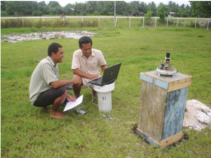
Installation of tipping-bucket rain gauge on Funafuti, Tuvalu
