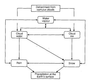
**Figure 4.1:** Diagram illustrating prognostic variables in a cloud microphysics scheme, and the processes that affect them.
