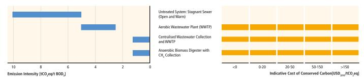
Figure 10.20 | Indicative CO<sub>2</sub>eq emission intensities and levelized cost of conserved carbon of different wastewater treatments (for underlying data and methodology, see Annex III).
