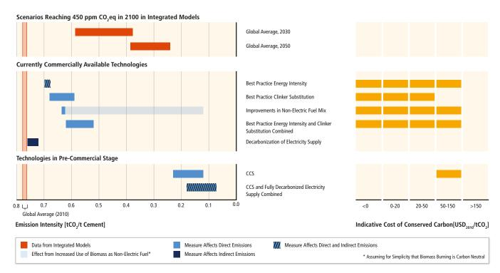
Figure 10.7 | Indicative CO<sub>2</sub> emission intensities and levelized cost of conserved carbon in cement production for various production practices/technologies and in 450 ppm scenarios of selected models (AIM, DNE21+, IEA ETP 2DS) (for data and methodology, see Annex III).
