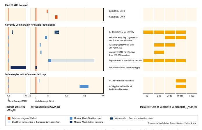
Figure 10.9 | Indicative global indirect (left) and direct (right) CO<sub>2</sub>eq emissions and levelized cost of conserved carbon resulting from chemicals production for various production practices/technologies and CO<sub>2</sub> emissions in IEA ETP 2DS scenario (for data and methodology, see Annex III).
