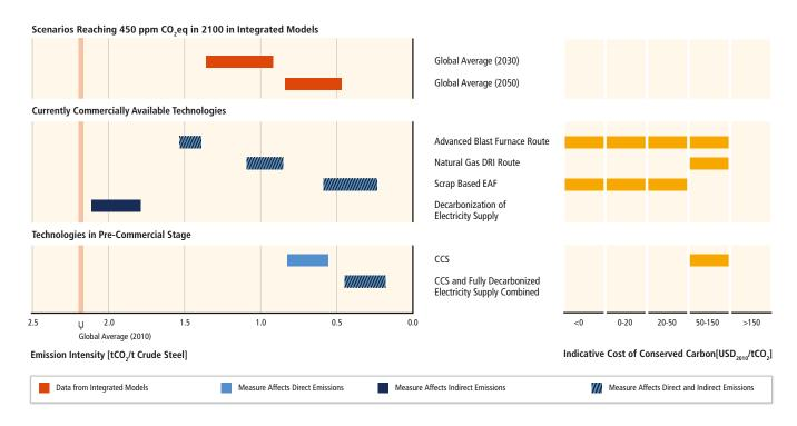
Figure 10.8 | Indicative CO<sub>2</sub> emission intensities and levelized cost of conserved carbon in steel production for various production practices/technologies and in 450 ppm scenarios of selected models (AIM, DNE21+, and IEA ETP 2DS) (for data and methodology, see Annex III).
