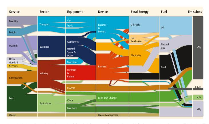
Figure 10.1 | A Sankey diagram showing the system boundaries of the industry sector and demonstrating how global anthropogenic emissions in 2010 arose from the chain of technologies and systems required to deliver final services triggered by human demand. The width of each line is proportional to GHG emissions released, and the sum of these widths along any vertical slice through the diagram is the same, representing all emissions in 2010 (Bajželj et al., 2013).
