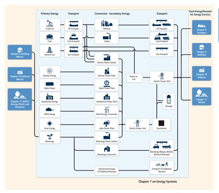
Figure 7.1 | Illustrative energy supply paths shown in order to illustrate the boundaries of the energy supply sector as defined in this report. The self-generation of heat and power in the end-use sectors (i. e., transport, buildings, industry, and Agriculture, Forestry, and Other Land Use (AFOLU)) is discussed in Chapters 8–11.
