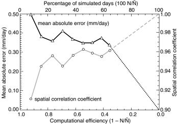
**Figure 10.17:** Similarity of time mean precipitation distributions obtained in a continuous RCM simulation and through statistical-dynamical downscaling (SDD) for different levels of disaggregation. Black line: mean absolute error (mm/day), grey line: spatial correlation coefficient. Horizontal axis: computational load of SDD. N is the number of days simulated in SDD, Ñ the number of days simulated with the continuous RCM simulation.
