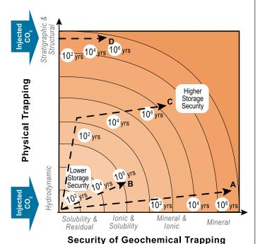
**Figure 5.10** Storage expressed as a combination of physical and geochemical trapping. The level of security is proportional to distance from the origin. Dashed lines are examples of million-year pathways, discussed in Box 5.4.
