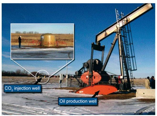
Figure 5.23 Typical CO, field operation setup: Weyburn surface facilities.
