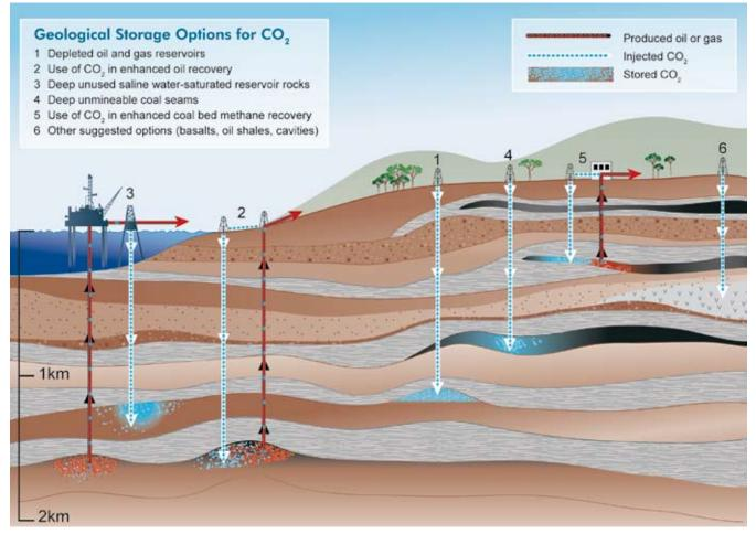
Figure 5.3 Options for storing CO, in deep underground geological formations (after Cook, 1999).
