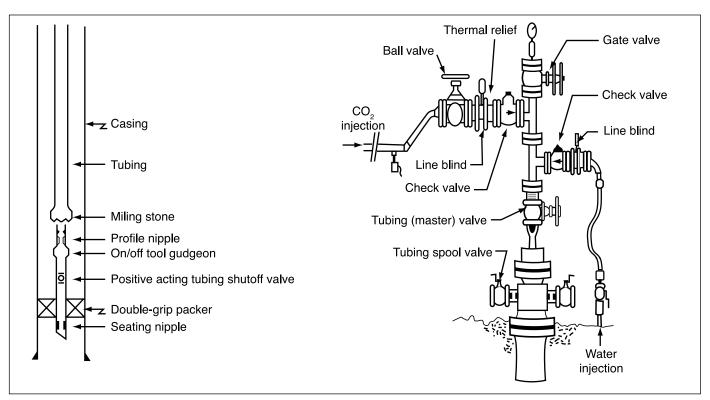
Figure 5.20 Typical CO<sub>2</sub> injection well and wellhead configuration.
