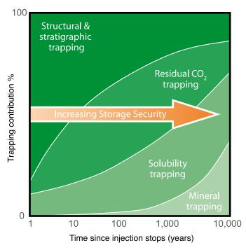
**Figure 5.9** Storage security depends on a combination of physical and geochemical trapping. Over time, the physical process of residual CO<sub>2</sub> trapping and geochemical processes of solubility trapping and mineral trapping increase.
