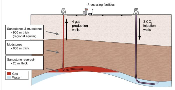
**Figure 5.5** Schematic of the In Salah Gas Project, Algeria. One MtCO<sub>2</sub> will be stored annually in the gas reservoir. Long-reach horizontal wells with slotted intervals of up to 1.5 km are used to inject CO<sub>2</sub> into the water-filled parts of the gas reservoir.
