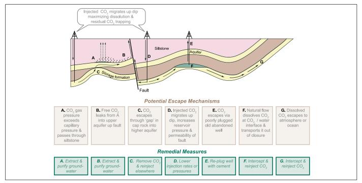
Figure 5.25 Some potential escape routes for CO<sub>2</sub> injected into saline formations.
