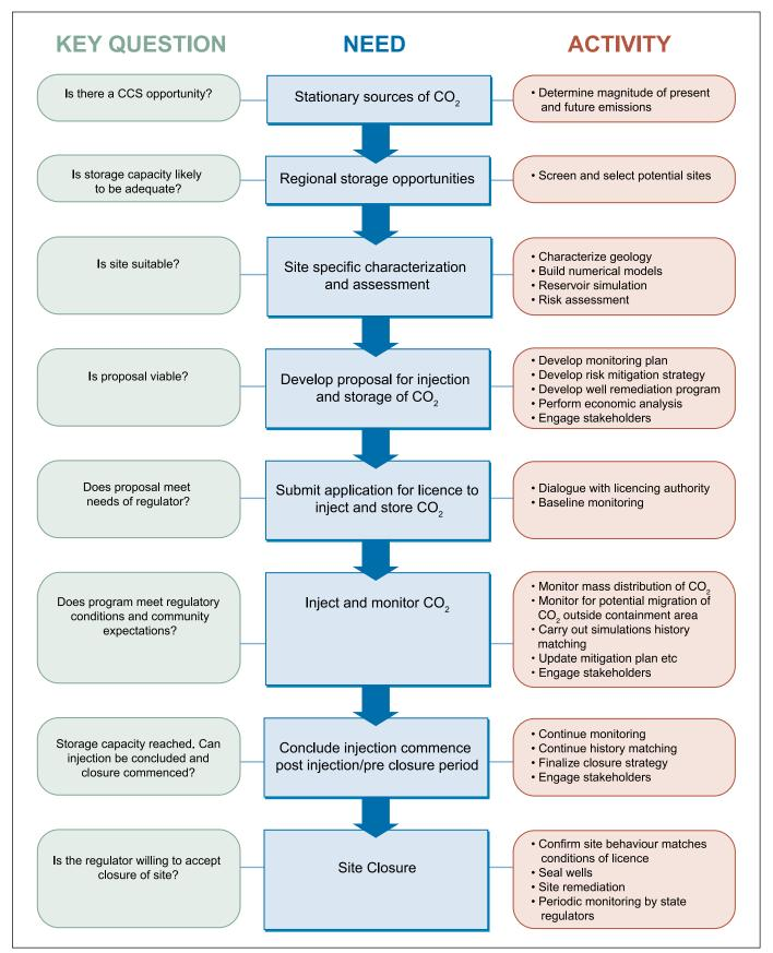
Figure 5.19 Life cycle of a CO<sub>2</sub> storage project showing the importance of integrating site characterization with a range of regulatory, monitoring, economic, risking and engineering issues.
