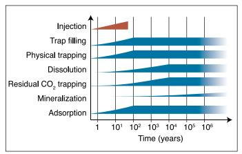
**Figure 5.18** Schematic showing the time evolution of various CO<sub>2</sub> storage mechanisms operating in deep saline formations, during and after injection. Assessing storage capacity is complicated by the different time and spatial scales over which these processes occur.
