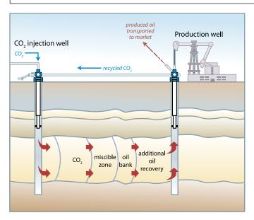
**Figure 5.15** Injection of  $CO_2$  for enhanced oil recovery (EOR) with some storage of retained  $CO_2$  (after IEA Greenhouse Gas R&D Programme). The  $CO_2$  that is produced with the oil is separated and reinjected back into the formation. Recycling of produced  $CO_2$  decreases the amount of  $CO_2$  that must be purchased and avoids emissions to the atmosphere.
