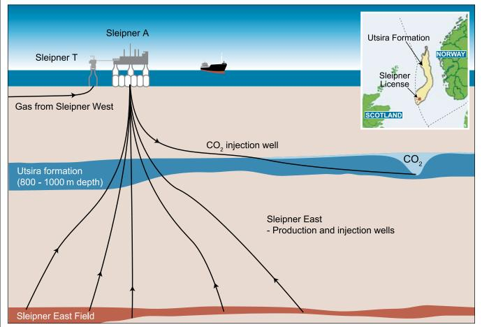
Figure 5.4 Simplified diagram of the Sleipner CO<sub>2</sub> Storage Project. Inset: location and extent of the Utsira formation.
