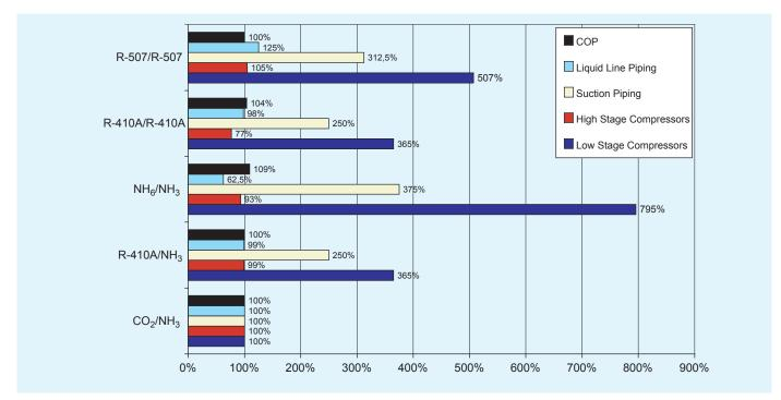
**Figure 4.1.** COP and size comparison of different components for different refrigerant combinations ( $Q_0 = 600 \text{ kW}$ ,  $t_c = 35^{\circ}\text{C}$ ;  $t_0 = -54^{\circ}\text{C}$ ;  $\text{CO}_2/\text{NH}_3$ -cascade system is equal to 100 %) (Roth and König, 2002).
