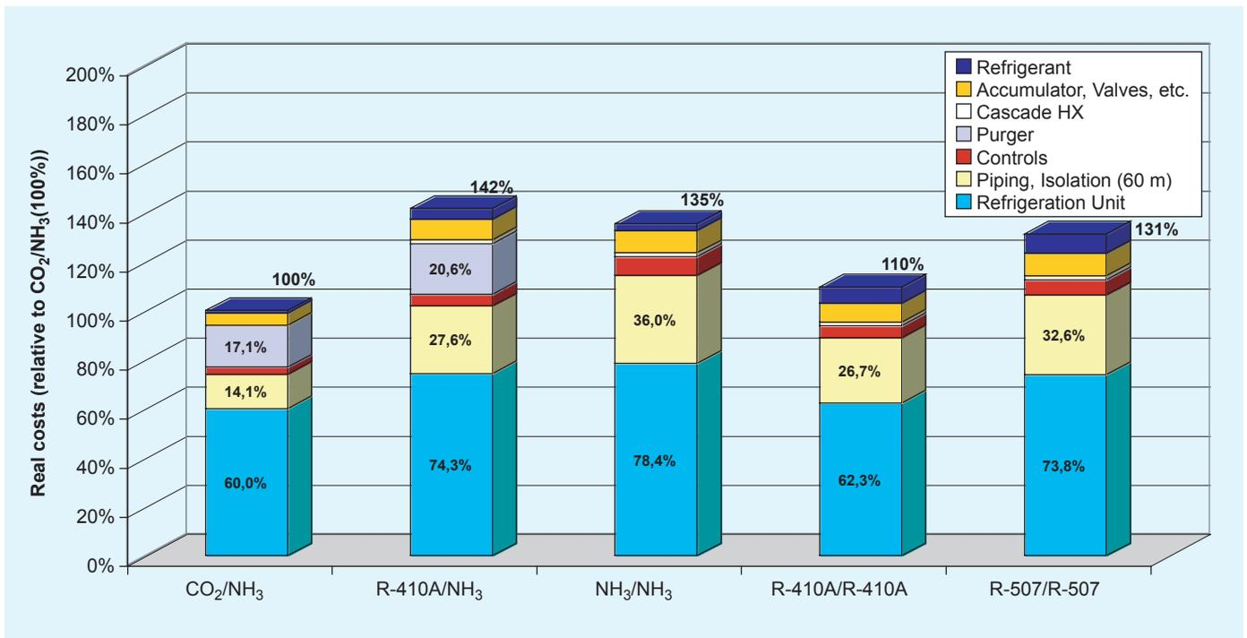
**Figure 4.2.** Cost comparison for different refrigerant combinations ( $Q_0 = 600 \text{ kW}$ ,  $t_c = 35^\circ\text{C}$ ;  $t_0 = -54^\circ\text{C}$ ;  $\text{CO}_2/\text{NH}_3$ -cascade system is equal to 100 %) (Roth and König, 2002).
