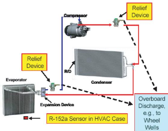
Figure 6.8. Direct HFC-152a System with Safety System.
