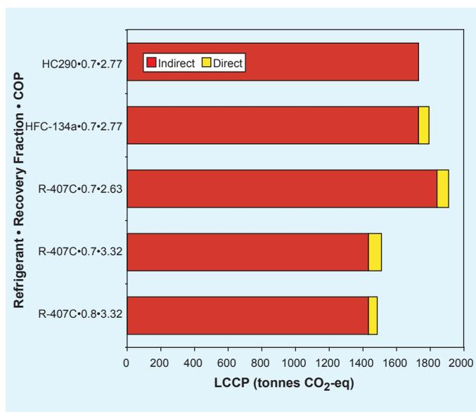
**Figure 5.9.** LCCP values for 355 kW air-cooled screw chillers in Japan for HFC-134a, R-290, and R-407C, with end-of-life refrigerant recovery of 70% or 80%, and COPs of 2.63, 2.77, or 3.32 (Onishi *et al.*, 2004).
