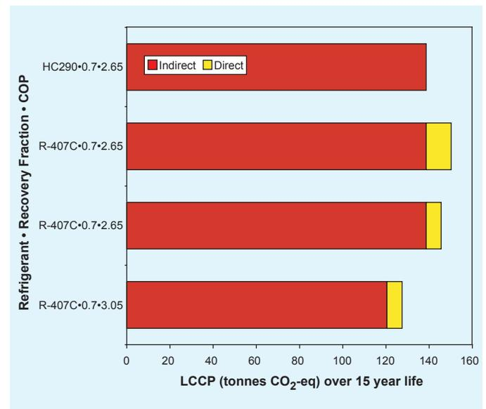
**Figure 5.8.** LCCP values for air-cooled 25 kW scroll chiller/heat pumps in Japan for R-290 and R-407C, with end-of-life recovery of 70% or 50% of the refrigerant charge, and with a system COP of 2.65 or 3.05 (Onishi *et al.*, 2004).
