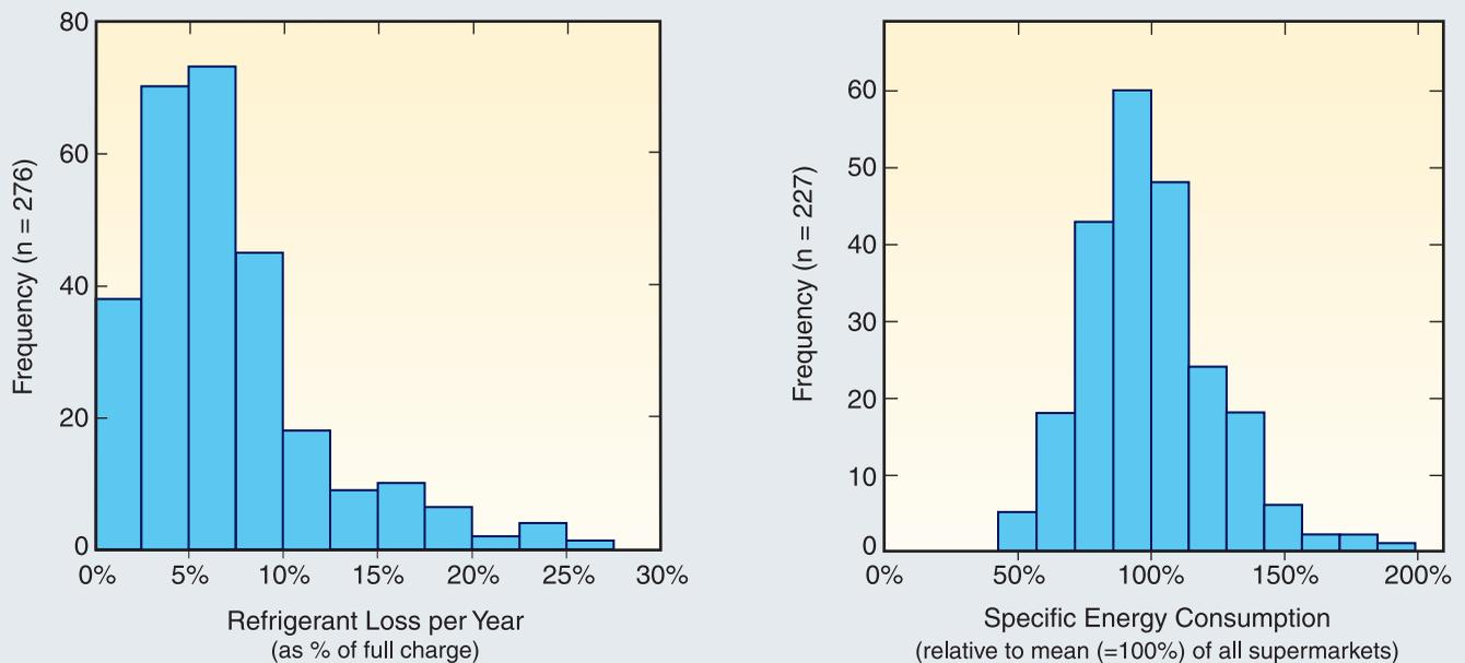
**Figure TS-10.** Variance of direct and indirect emissions within equipment populations. Annual leakage rates of mobile air conditioning systems in a fleet of passenger vehicles (left panel, n=276). Specific energy consumptions expressed as percentage of the mean for a group of standard layout supermarket refrigeration units (right panel, n=227).
