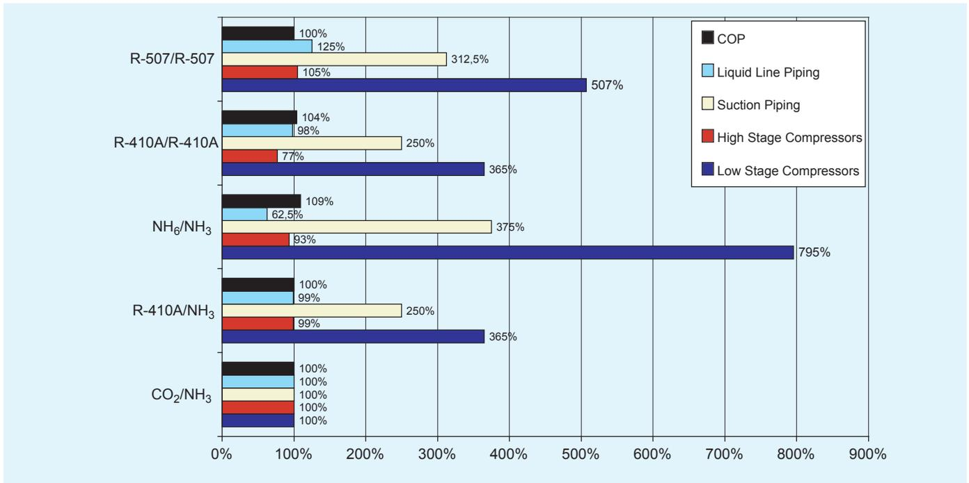
**Figure 4.1.** COP and size comparison of different components for different refrigerant combinations ( $Q_0 = 600 \text{ kW}$ ,  $t_c = 35^\circ\text{C}$ ;  $t_0 = -54^\circ\text{C}$ ;  $\text{CO}_2/\text{NH}_3$ -cascade system is equal to 100 %) (Roth and König, 2002).
