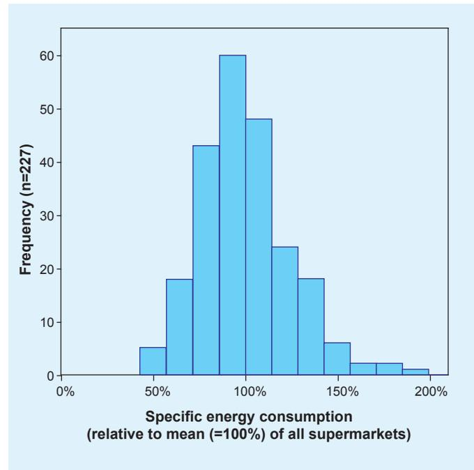
**Figure 3.3.** Distribution of measured specific energy consumptions (originally expressed as kWh d<sup>-1</sup> m<sup>-1</sup> of cooled display cases) expressed as percentage of the mean for 227 standard stores using standard HFC technology of a German supermarket chain – after Harnisch *et al.* (2003).
