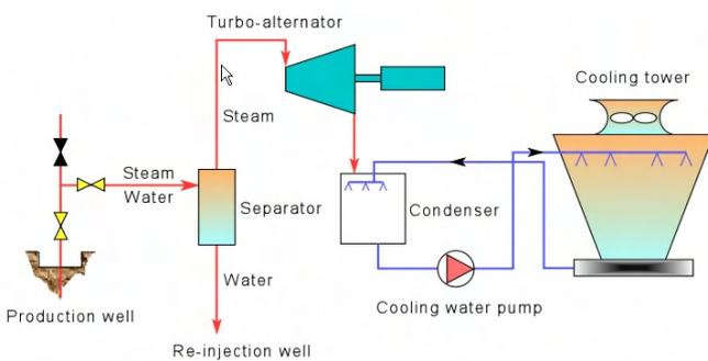
**Figure 7. A schematic diagram of a geothermal condensing power plant**
