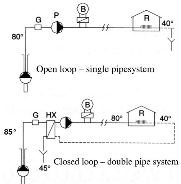
**Figure 10. Two main types of district heating systems.** G=gas separator, P=pump, B=boiler, R=radiation heating, HX=heat exchanger (Dickson and Fanelli, 2003).
