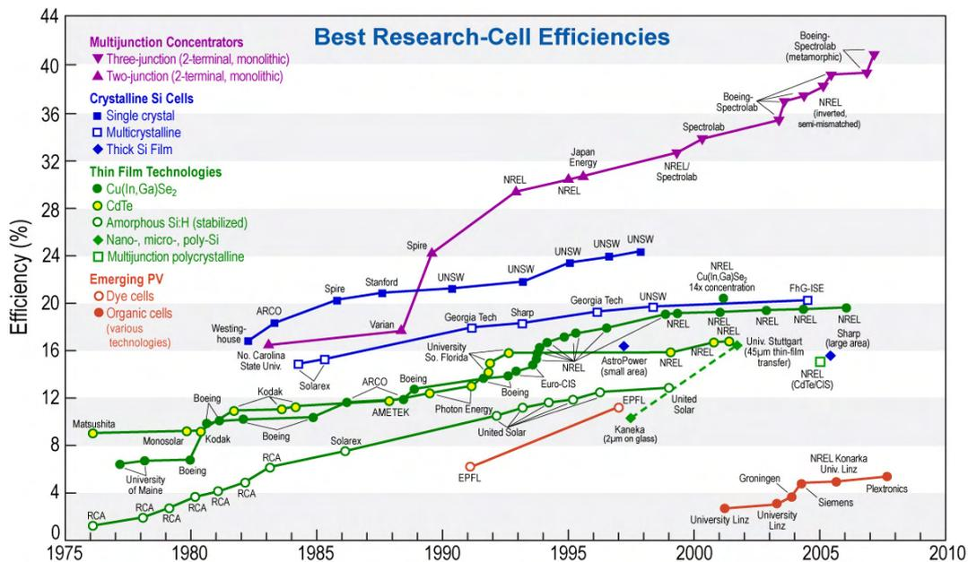
Figure 15. Improvements in conversion efficiencies for various technologies of laboratory photovoltaic cells (compiled by L.L. Kazmerski, NREL).
