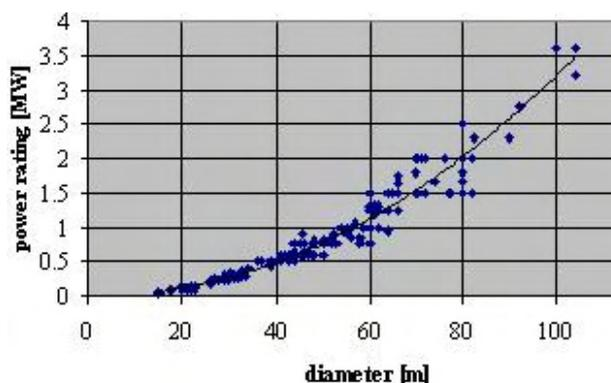
**Figure 2. Rating vs diameter of wind turbine designs**
