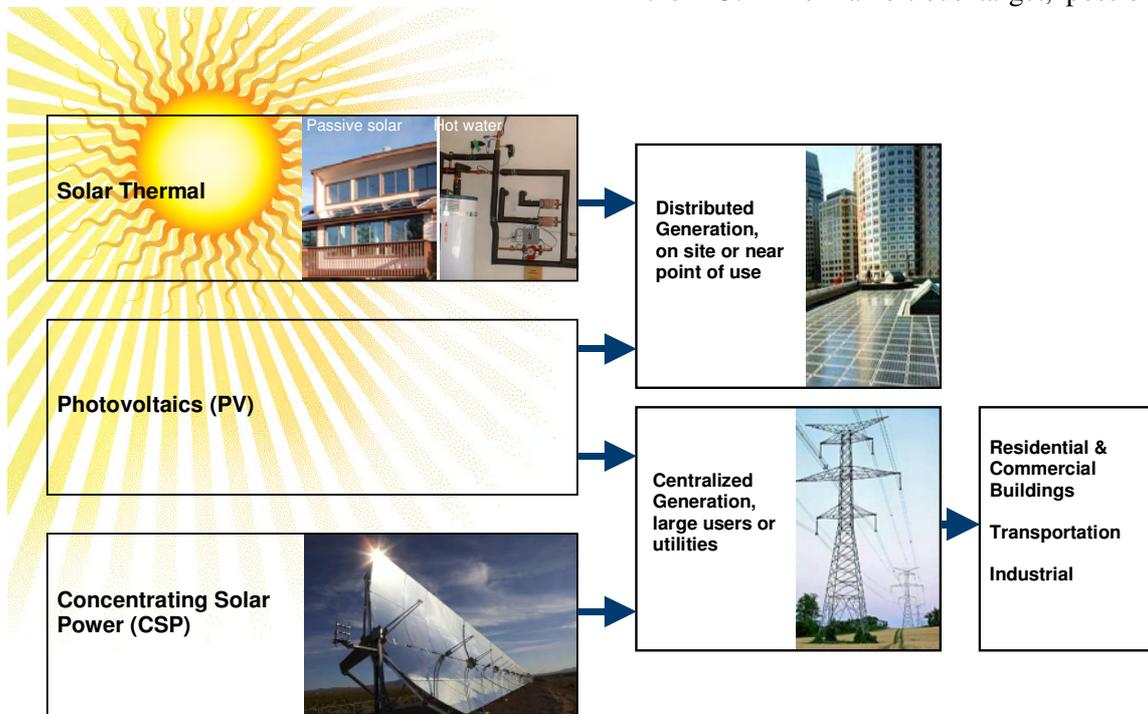
Figure 3. The solar resource can be used by direct solar technologies to supply thermal energy and electricity to end-users in the buildings, transportation, and industrial sectors
