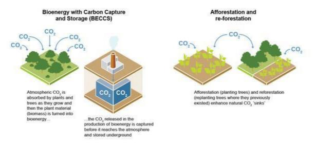
**FAQ4.2, Figure 1:** Carbon Dioxide Removal (CDR) refers to the process of removing  $CO_2$  from the atmosphere. There a number of CDR techniques, each with different potential for achieving 'negative emissions', as well as different associated costs and side effects.
