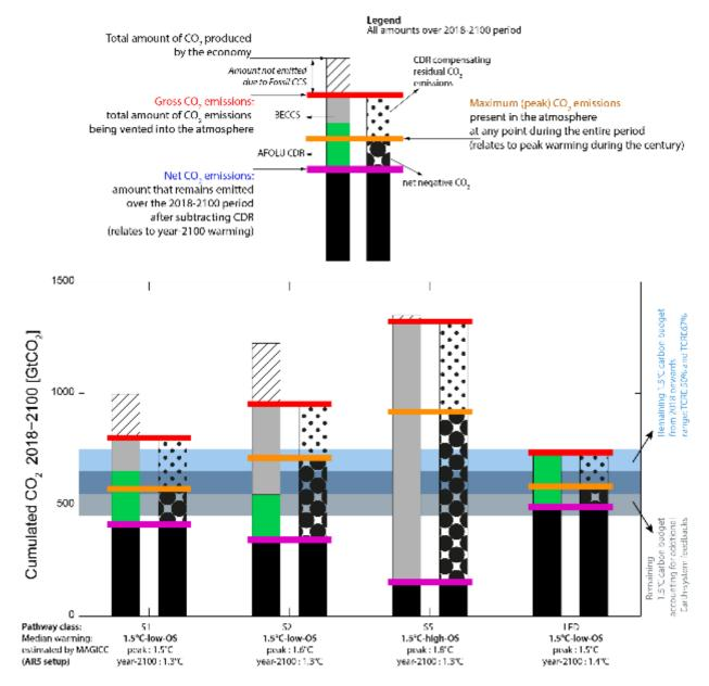
**Figure 2.10:** Accounting of cumulative CO<sub>2</sub> emissions for the four 1.5°C-consistent pathway archetypes. See top panel for explanation of the barplots. Total CDR is the difference between gross (red horizontal bar) and net (purple horizontal bar) cumulative CO<sub>2</sub> emissions over the period 2018–2100. Total CDR is the sum
